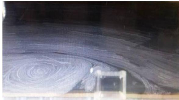
Figure 1: Flow Modification by Vertical wall Abutment (Flow is from Right to Left)
