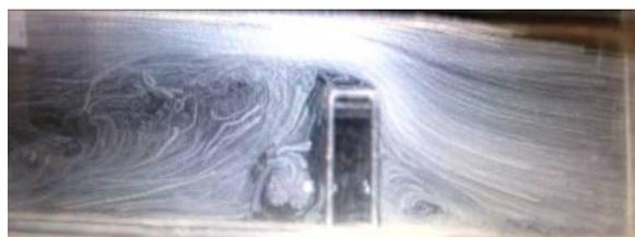
(c) Vertical Wall Abutment (Model No. 3)
