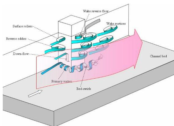
**Figure 8: Flow Structures around an Abutment**
