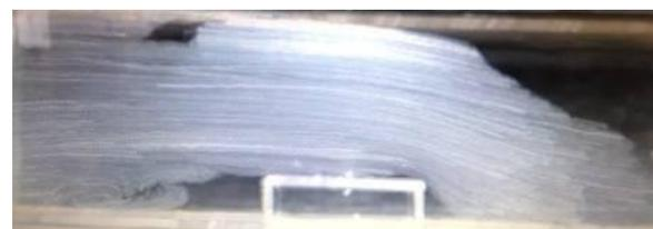
(c) Vertical Wall Abutment (Model No. 5)
