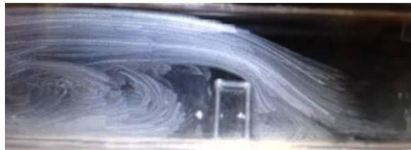
(b) Vertical Wall Abutment (Model No. 2)
