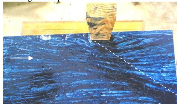
**Figure 7: Wet Paint Impressions around Vertical Wall Abutment (L = 26mm and W = 60mm, Re = 10000)**
